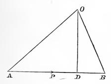
52. Definition of the moment of a force. Let AB represent any force P and let () be any point in the same plane. From O let fall a perpendicular OD on AB. Then AB.OD or P.OD is called the moment of P about the point O. Hence we have the following definition:
